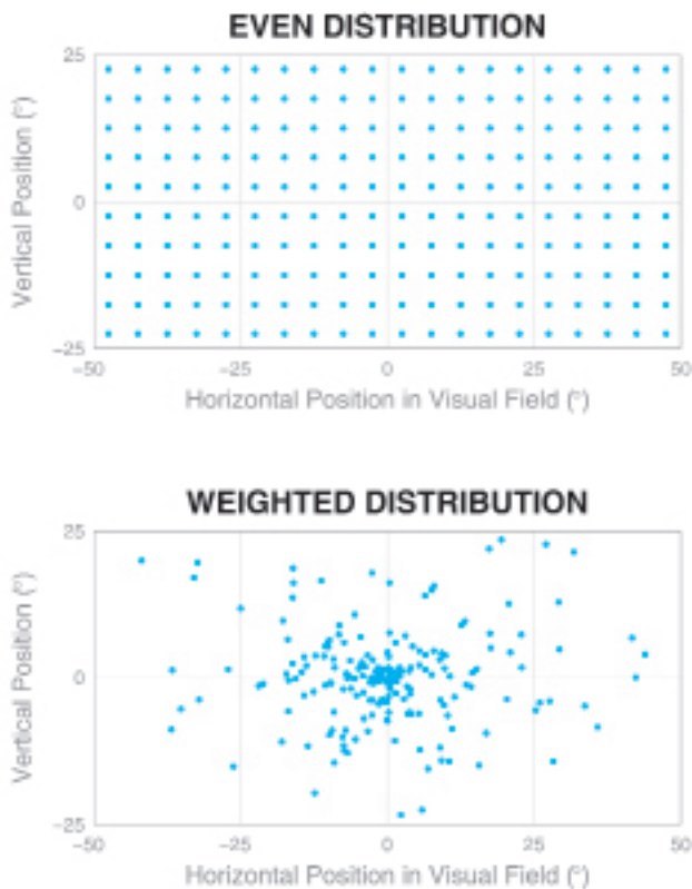
Fig. 3. Charts showing simulated phosphene distribution patterns. Vertical and horizontal axes represent the positions along the visual field, and each dot represents a phosphene from an independent electrode contact. While there are equal numbers of contacts in the 2 diagrams, the lower pattern matches the intrinsic acuity profile of the primate visual system, and has a much higher focal acuity than the upper pattern. Upper : When prosthesis electrode contacts are placed on the retina in a regular pattern, the generated phosphenes also appear in a regular pattern across the visual field. Lower : When contacts are placed in a physically regular pattern in tissue downstream of the retina, the phosphenes will appear in a pattern strongly weighted to the center of the visual field.
